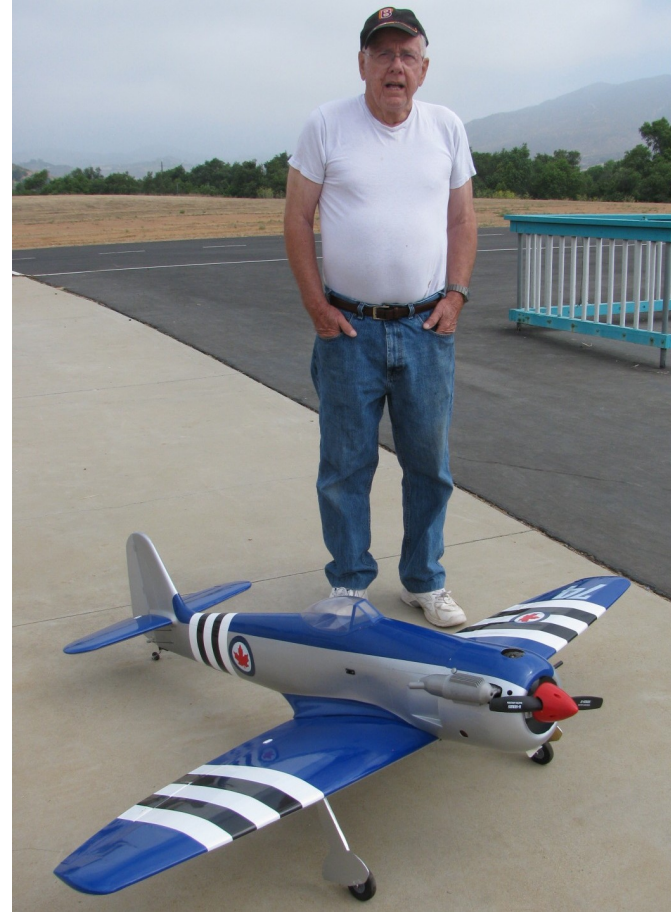
Bill Demore has a new Sea Fury ARF from Will Hobby that had a successful maiden flight. It has a wingspan of 66 in. and weighs 11.5 lbs. It is powered by a Magnum 91 two-stroke glow engine running a 14 x 6 Master Airscrew prop.
