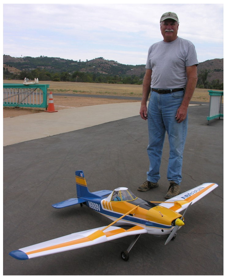
Greg LaVay is flying this Cessna AG Wagon crop duster ARF from Discount Hobbies. It is powered by an OS-AX-75 two-stroke glow engine running a 14 x 6 prop. The wingspan is 74 in. and it weighs 12--13 lbs.
