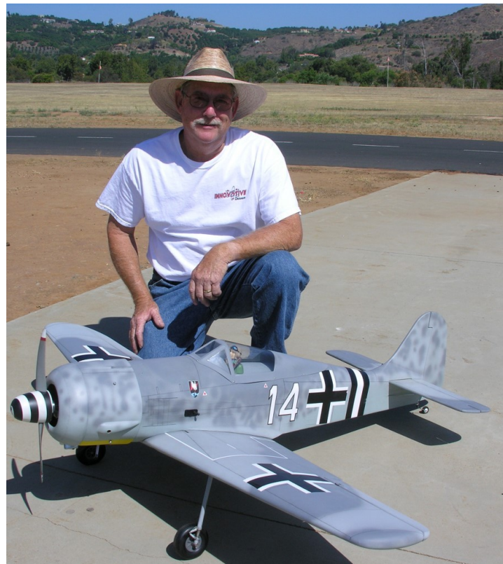
Joe Villarreal is flying this FW-190 Focke Wulf ARF from H. & M. Performance. It is powered by a Saito 100 four-stroke glow engine. The wingspan is 63 in. and it has a 29.5 oz. wing loading. It weighs 9 lbs. 4 oz. and has electric retracts.
