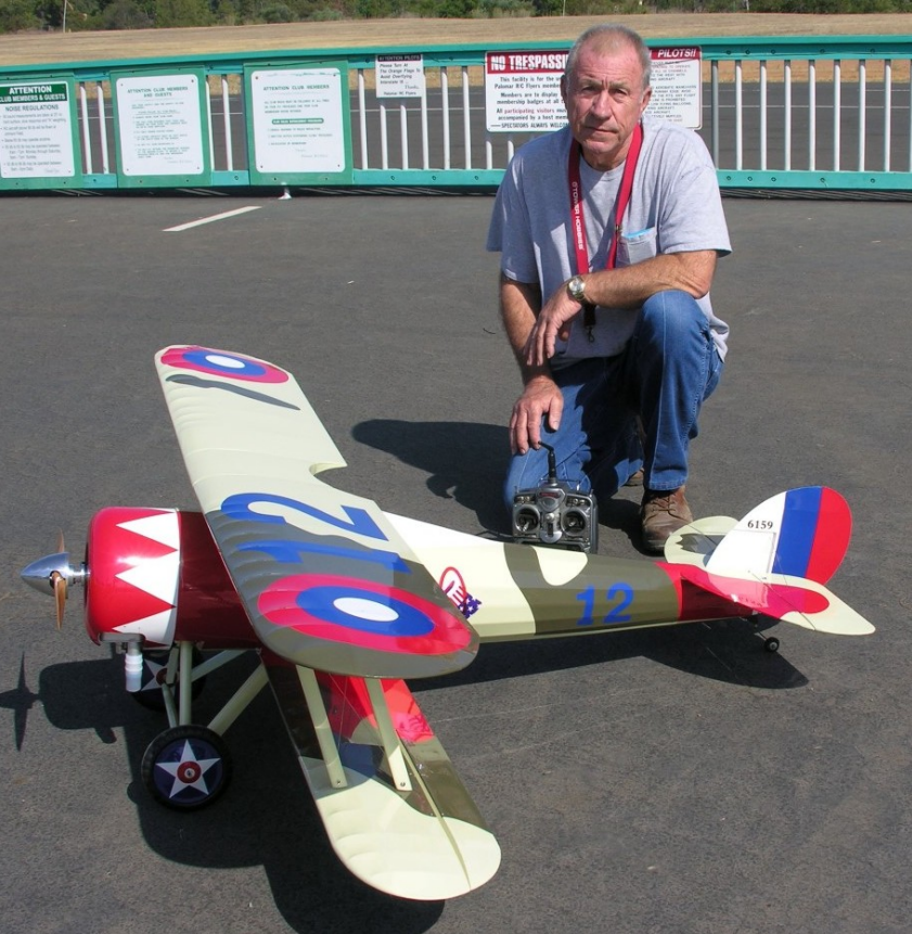
Jim Truett had a successful maiden flight with his new bi-plane Nieuport 28 from Maxford USA. It is powered by a DLE-30cc gas engine running a Xoar 18 x 8 prop. The wingspan is 70 in., wing area is 1165 sq. in. and the length is 56 in. It weighs 13.5 lbs.
