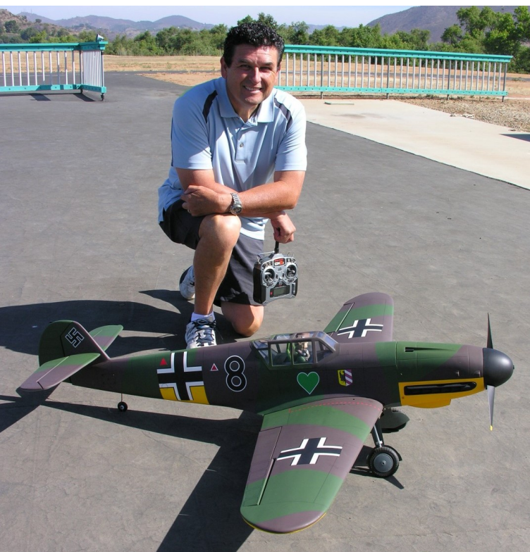
Pancho Castillo has a new ME-109 Messerschmitt ARF from Hangar 9. It has an E-flite 60 size electric motor, Castle Creations 80 amp ESC, with a 6 cell 22.2 volt 5000 mAh battery, and electric retracts. The wingspan is 63 in. and it weighs 11 lbs.
