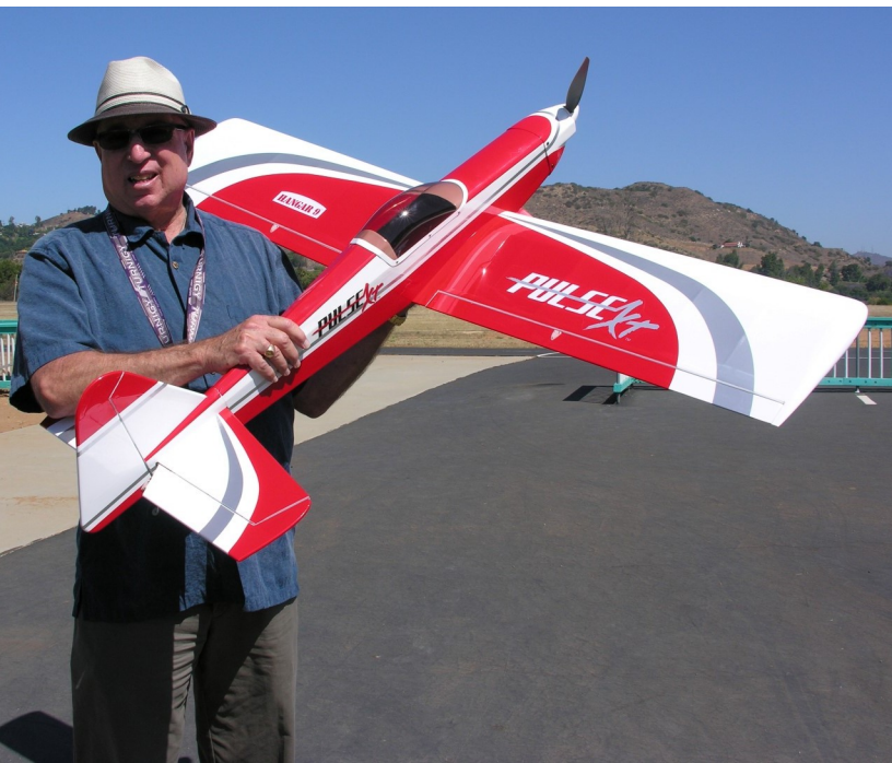
Roy DeMille had a successful maiden flight with his new ARF Pulse XT from Hangar 9. It has a wingspan of 65 in. and length is 23 in. It has an electric power 46 motor, 60 amp ESC, 4000 mAh 14.8 volt battery, and it weighs 9.5 lbs. Roy is also flying this new Apprentice from E-flite. The wingspan is 58 in. and it is 37 in. long. It has an 8040 kv electric motor, 30 amp ESC, and 3200 mAh 11.1 volt battery. It also comes with a Spektrum DX-5E transmitter.
