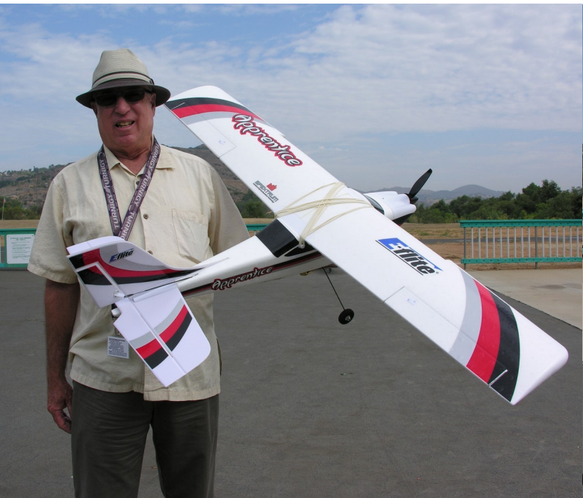
Roy DeMille had a successful maiden flight with his new ARF Pulse XT from Hangar 9. It has a wingspan of 65 in. and length is 23 in. It has an electric power 46 motor, 60 amp ESC, 4000 mAh 14.8 volt battery, and it weighs 9.5 lbs. Roy is also flying this new Apprentice from E-flite. The wingspan is 58 in. and it is 37 in. long. It has an 8040 kv electric motor, 30 amp ESC, and 3200 mAh 11.1 volt battery. It also comes with a Spektrum DX-5E transmitter.
