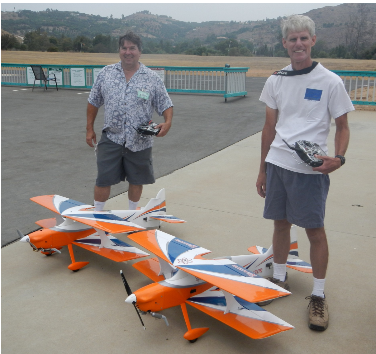
Ron Mason took this photo of Richard Martin and John Hartsell, Jr. on July 19, 2013. They are both flying a Great Planes Reactor Biplane. Wingspan is 50 something and power is a Saito 100 4 stroke.
