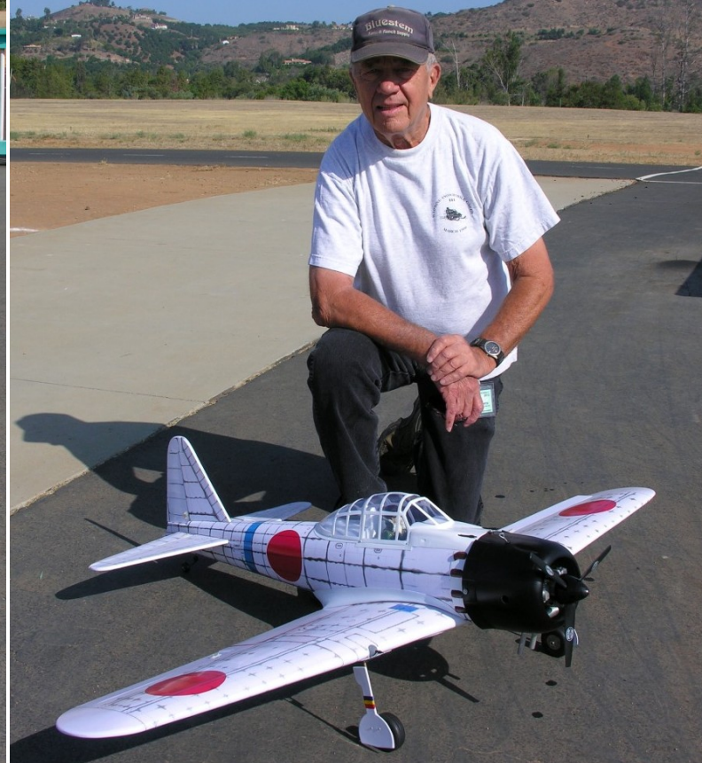
Paul Schubarth had a successful maiden flight with this new Zero from VQ Models in the Pearl Harbor Edition. It is powered by an OS-46-AX-II glow engine running a 3-blade Master Airscrew 10 x 7 prop. It has a Bisson exhaust with electric retracts from Hobby King. The wingspan is 60 in. and it weighs 6.5 lbs.
