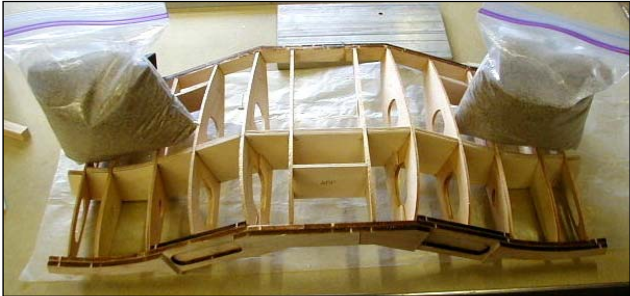
Gluing center section of gull wing.
