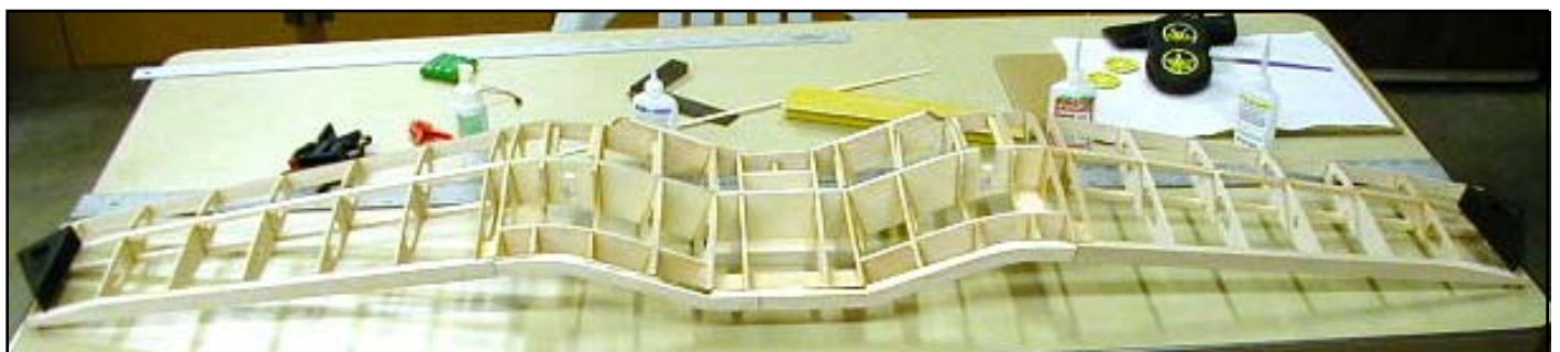
Left & right wing attached to center section.
