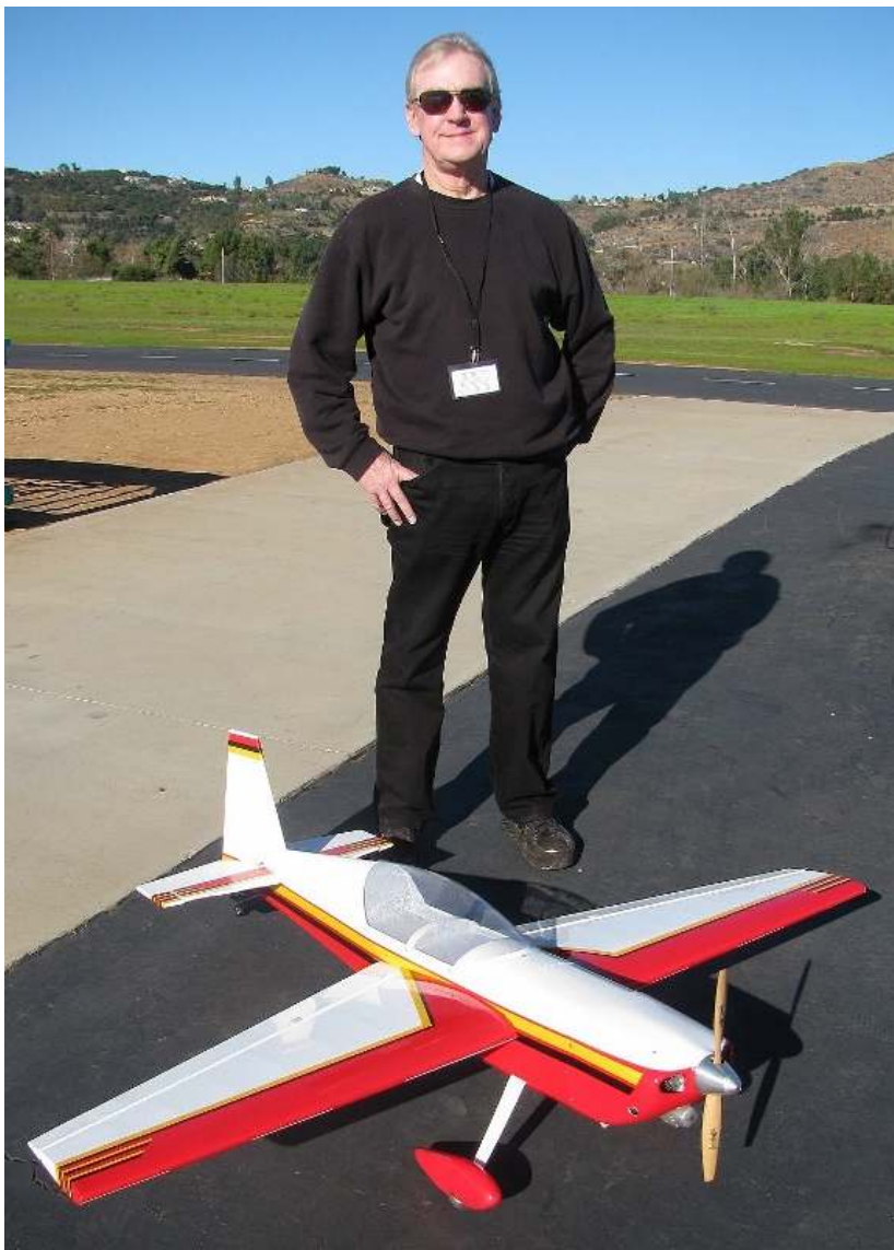
Steve Stuart is flying this new Edge 540 from Aeroworks. The wingspan is 60 in. It is powered by an OS-55 glow engine running a 12 x 6 prop.
