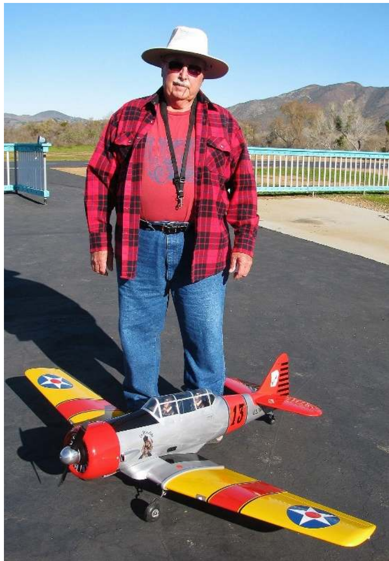
Frank Burke had a successful maiden flight with this new AT-6 Texan ARF from TopFlite. It has a 69 in. wingspan with a 30.2 oz. wing loading. It is powered by a Saito 100 four-stroke glow engine running a 14 x 7 prop. It has mechanical retracts and weighs 9.9 lbs.
