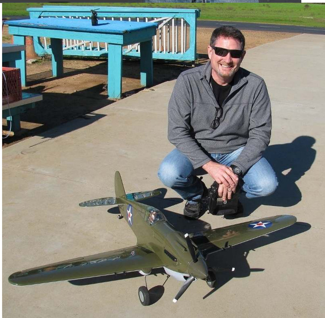
Dave Swaffer has a P-40 Warhawk with a 56 in. wing-span from Hangar 9. It has a Power 52 E-flite electric motor, E-flite 80 speed control, and 5S 4500 mAh battery.
