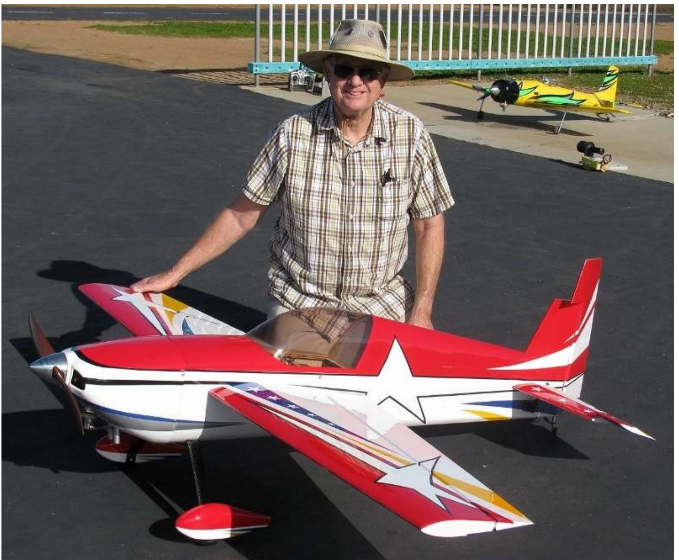
John Cutler made a successful maiden flight with his new A. J. Slick from 3D Hobby. It has a 71 in. wingspan. It is powered by a DLE-30cc gas engine running a Vess 20A prop. It has 7955 HiTec servos and he is using a 2 cell Lipo battery.
