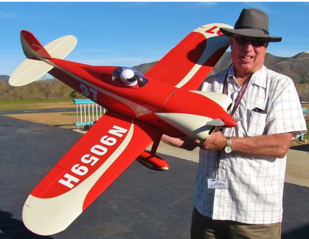
Steve Stuart is flying this new Edge 540 from Aeroworks. The wingspan is 60 in. It is powered by an OS-55 glow engine running a 12 x 6 prop.
