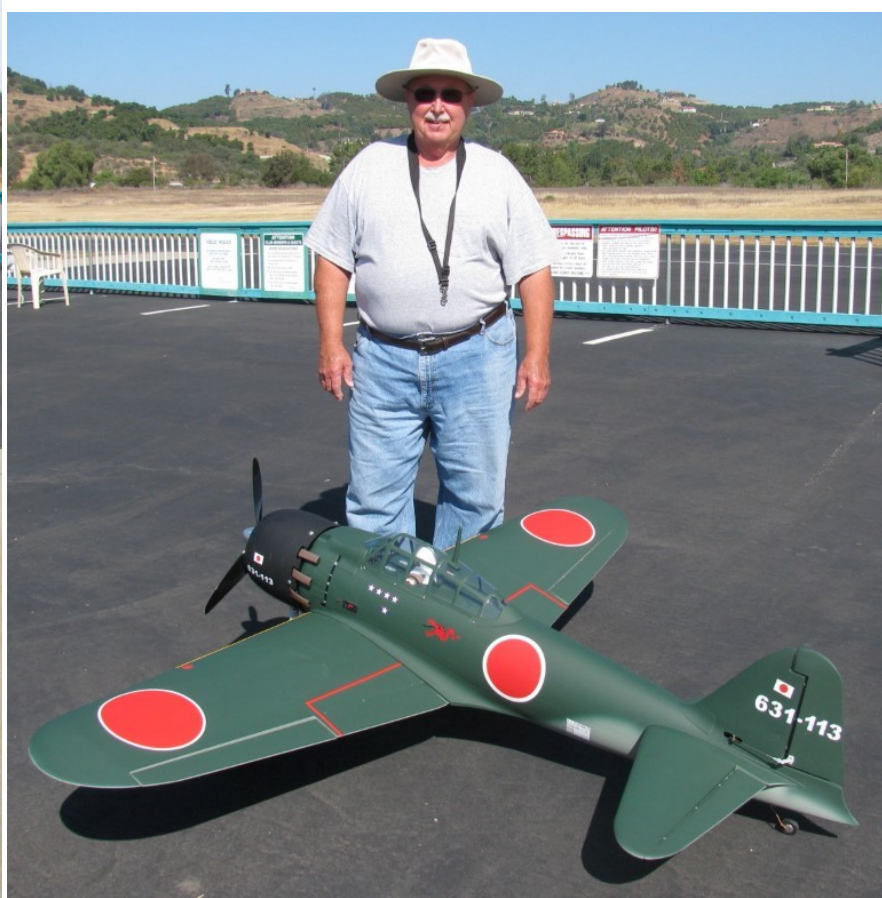
Frank Burke is flying this FW-190 Focke-Wulf ARF from KMP. It has a wingspan of 71 in. with a 43 oz. wing loading. It is powered by a Saito 180 glow engine with a 16 x 8 APC prop. It has Sierra retracts and weighs 16 lbs. 3 oz. Frank also flew a maiden flight with this new Zero ARF from CMP. It is powered by a DLE-55cc gas engine with rear exhaust running a 3-blade Biela 20 x 10 prop. The wingspan is 83 in. with a 46.5 oz. wing loading. It has Robart retracts and weighs 24 lbs. 15 ozs.
