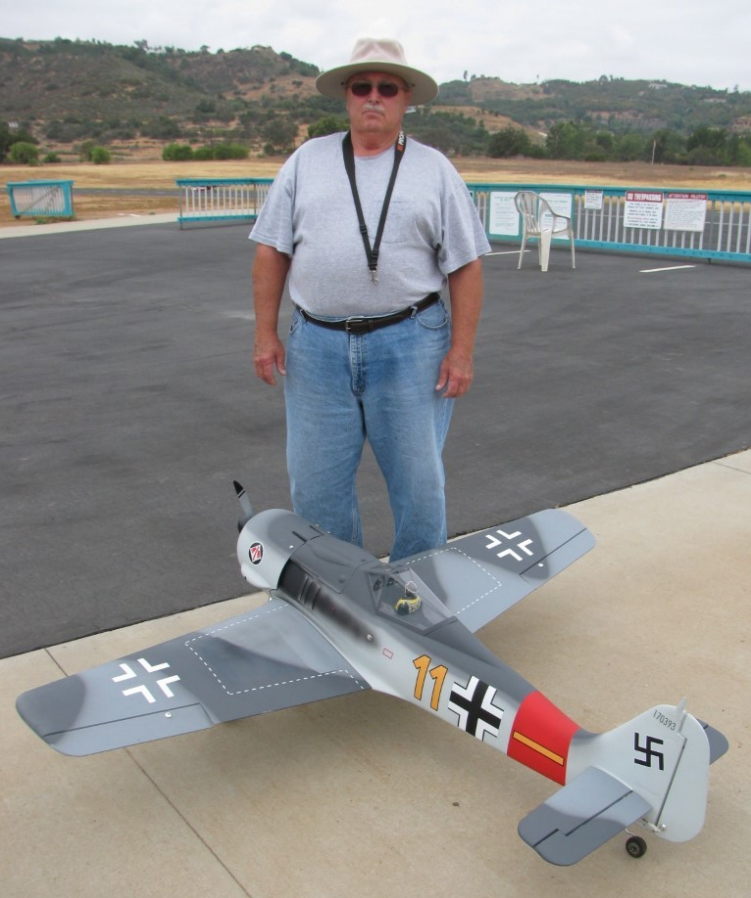
Frank Burke is flying this FW-190 Focke-Wulf ARF from KMP. It has a wingspan of 71 in. with a 43 oz. wing loading. It is powered by a Saito 180 glow engine with a 16 x 8 APC prop. It has Sierra retracts and weighs 16 lbs. 3 oz. Frank also flew a maiden flight with this new Zero ARF from CMP. It is powered by a DLE-55cc gas engine with rear exhaust running a 3-blade Biela 20 x 10 prop. The wingspan is 83 in. with a 46.5 oz. wing loading. It has Robart retracts and weighs 24 lbs. 15 ozs.
