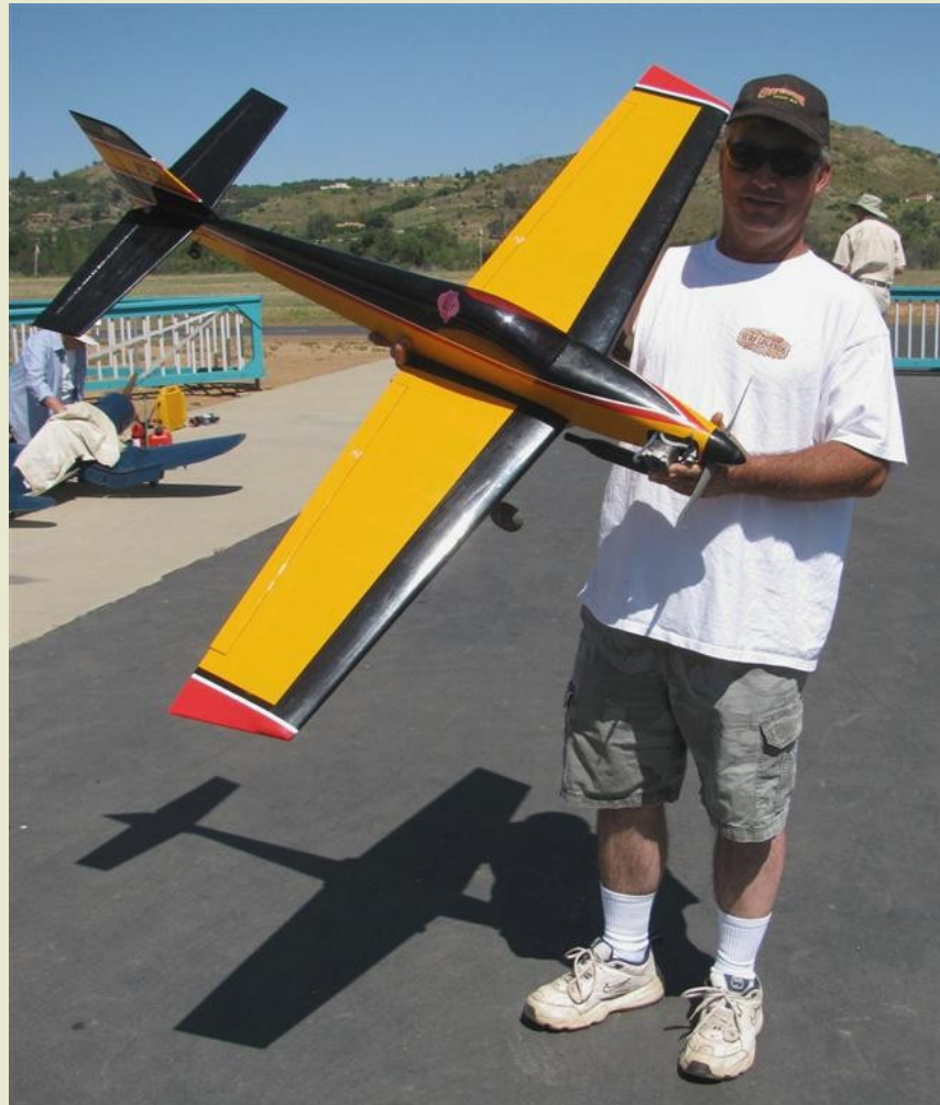
Scott Holmes is flying this Tsunami sport plane from Juno R/C Models. It is powered by a Magnum 46 two-stroke glow engine. The wing span is 58.5 in. and it weighs about 6 lbs.
