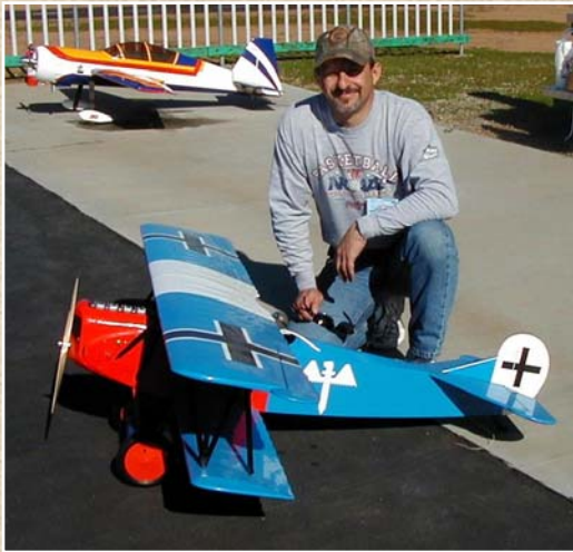
David Bracci was out at the field flying this Fokker DR 7 ARF from Hangar 9. It is a WWI biplane 60 size running with a Saito 82 4-stroke glow engine.
