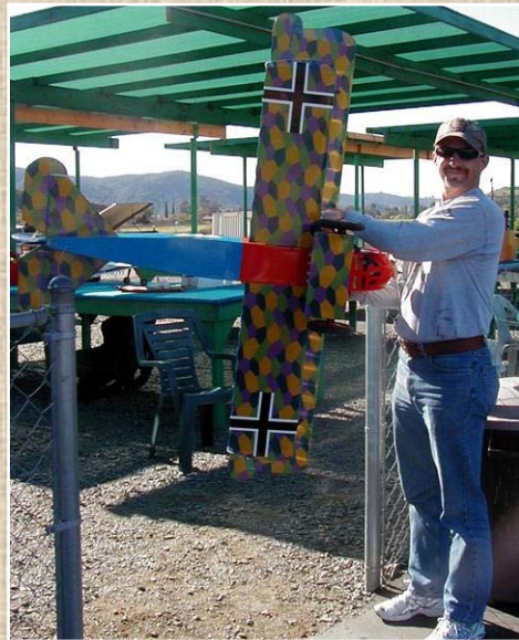
Jim Truett is also flying a WWI plane, the Blue Max ARF from Model Tech. It has a wing span of 67.25, total wing area is 756 sq. in., with fuselage length at 49.5, and weighing 5.5 - 6.5 lbs. Engine is a 4-stroke glow OS-52 and is piloted by Von Richthofen.
