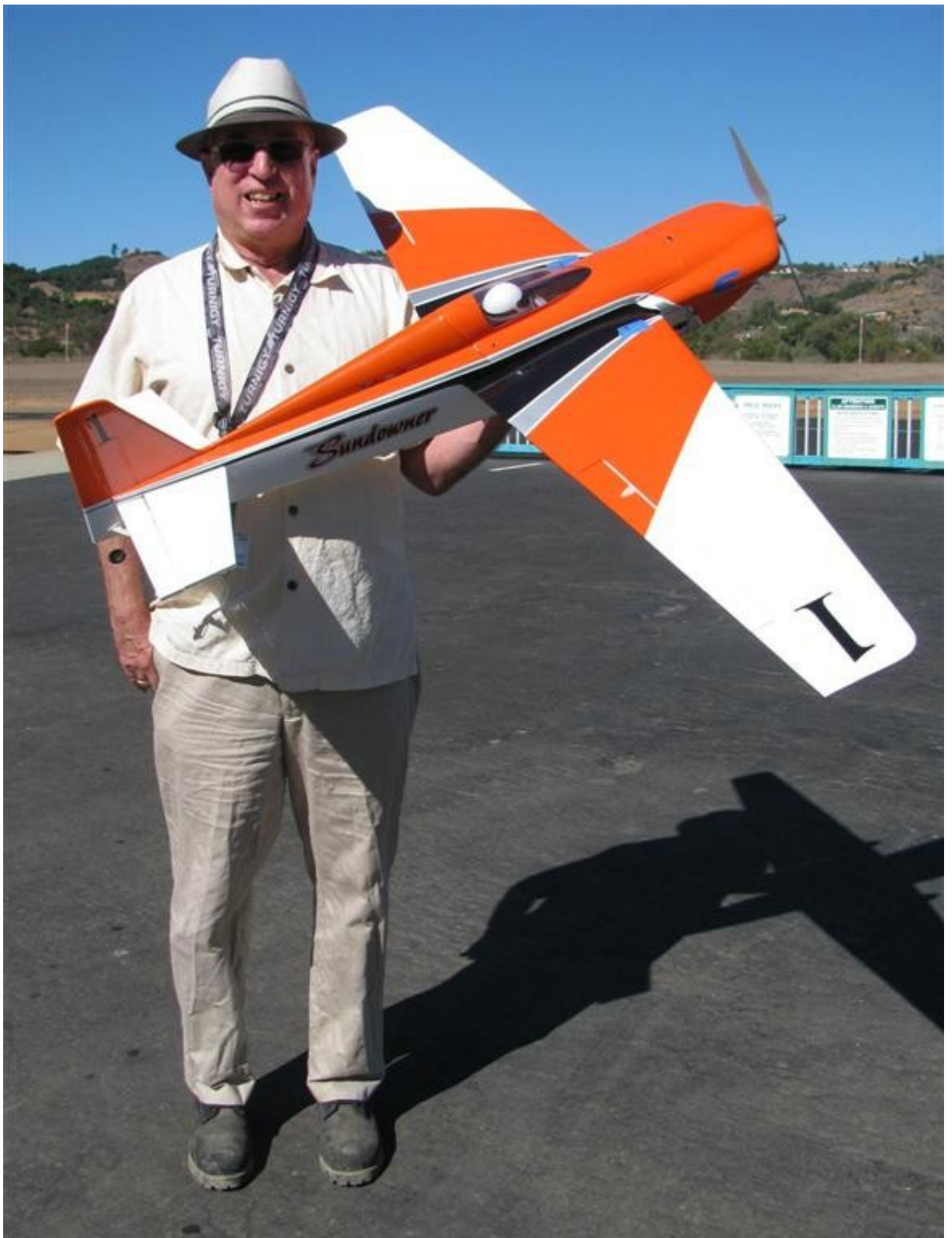
25 Roy DeMille has a new Sundowner from Hangar 9. The wingspan is 63 in. It has an E-flite power 46 electric motor, 60 amp ESC, 4000 mAh 4-cell 14.8 volt battery. Ethel Burke photo
