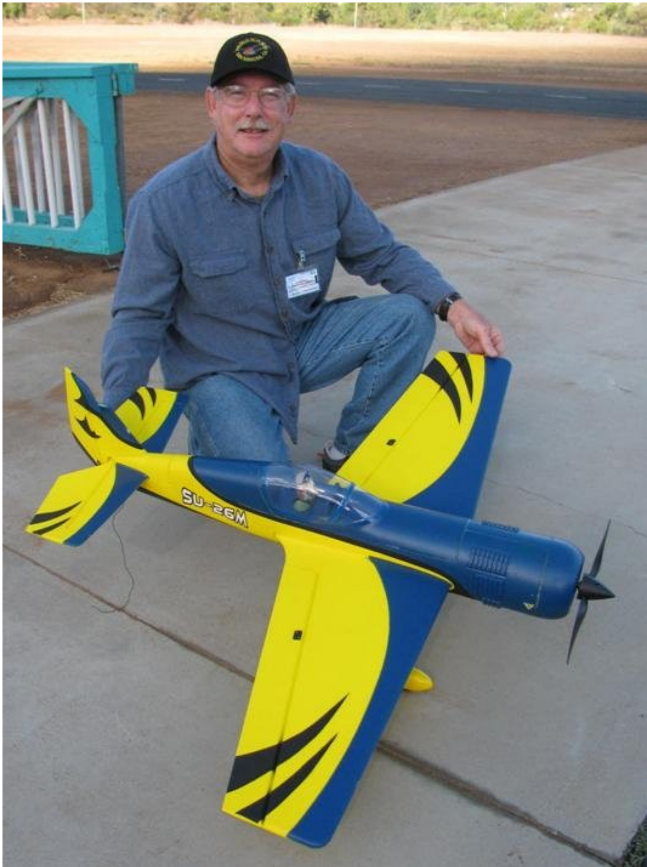
Joe Villarreal has a new Sukhoi foam SU-26M airplane with an electric motor from Dynam RC. It has a wingspan of 49 in. with a 2200 mAh 4-cell battery and it weighs 2.5 lbs. Ethel Burke Photo
