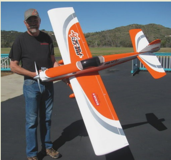
Eric Phillips has a new Pulse 125 from Hangar 9 with a wingspan of 76 in. It is powered by a Saito 125 four-stroke glow engine using an APC 15 X 6 prop.
