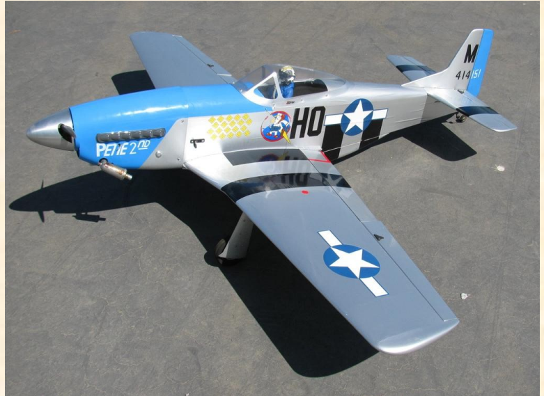
Isaac Edwards is flying a P-51 Mustang from World Models. It has a wing span of 65 in. and is powered by a Saito 91 four-stroke glow engine.
