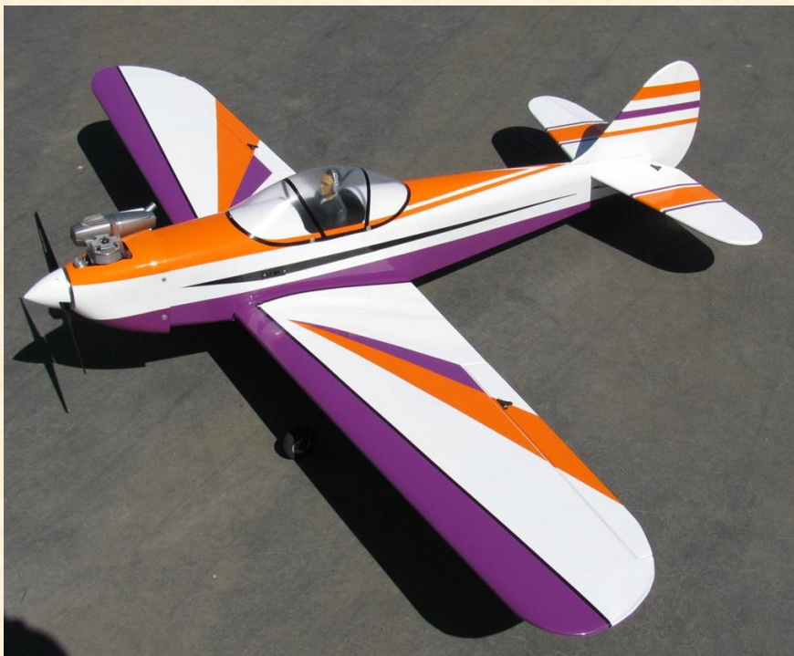
Robert Wylie brought out one of his smaller new planes that is a really good flyer. It is a Rambler 45 also from World Models. It has a 63 in. wing span and is powered by an OS-46 AX two-stroke glow engine.
