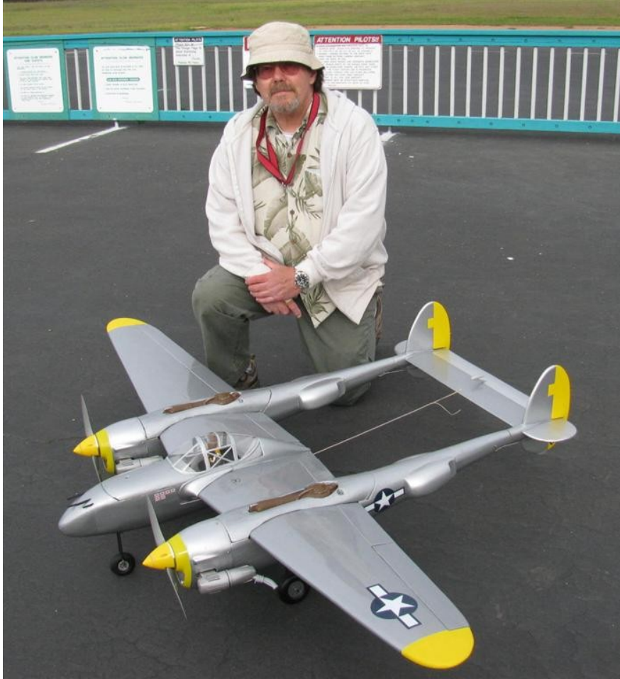
Ed Ramsey has built and flew this new twin-engine P-38 Lightning from a Royal Kit that is no longer available. It has a wingspan of 74 in. and includes flaps. It is powered by two OS-55 AX glow engines. It weighs 11 lbs. 4 oz. He has a removable tail section for transporting. Ethel Burke photos
