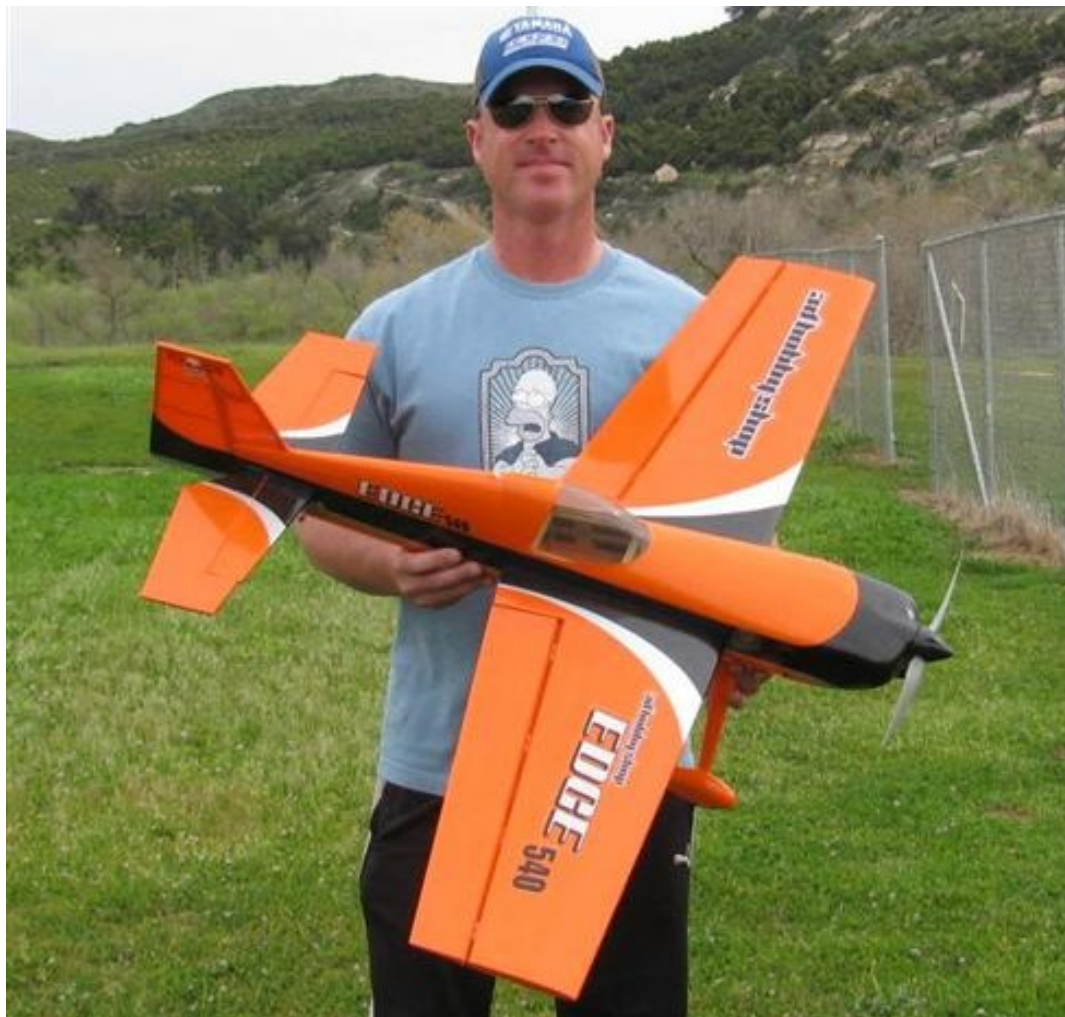
Gary Kaplan has a new electric Edge 540 from 3-D Hobby Shop. It has a wingspan of 41 in. and length is 39 in. He is using an Omega motor with 3S battery.
