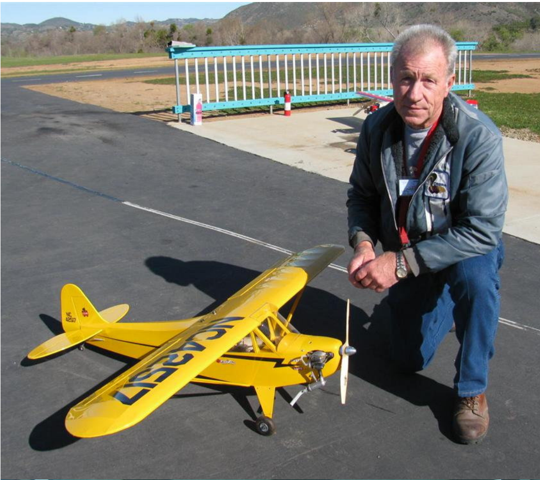
Jim Truett has built a new clip wing Piper Cub 40 from a Great Planes kit. It is covered with Ultracoat and weighs 7 lbs. with a wingspan of 61.5 in. It is powered by a Saito 82 four-stroke glow engine.
