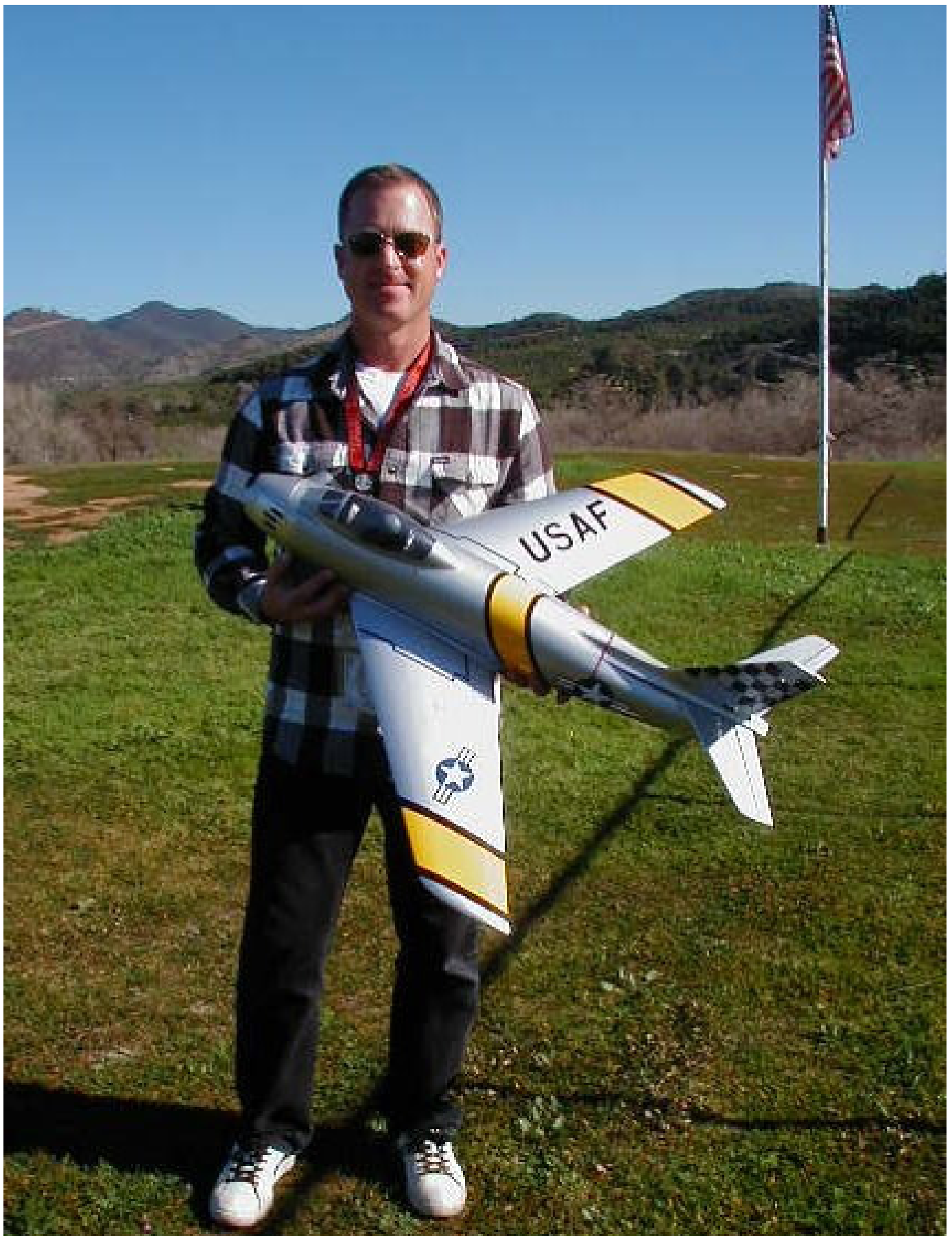
Gary Kaplan is flying this new F-86 Sabre Jet from E-flite. Plane has a fiberglass fuselage with balsa wings. The tri-landing gear has suspension oleo struts. It weighs 55 oz's. and has a wingspan of 33.8 in. and length of 35.4 in. It has a 3600 kv motor EDF and 4S battery.
