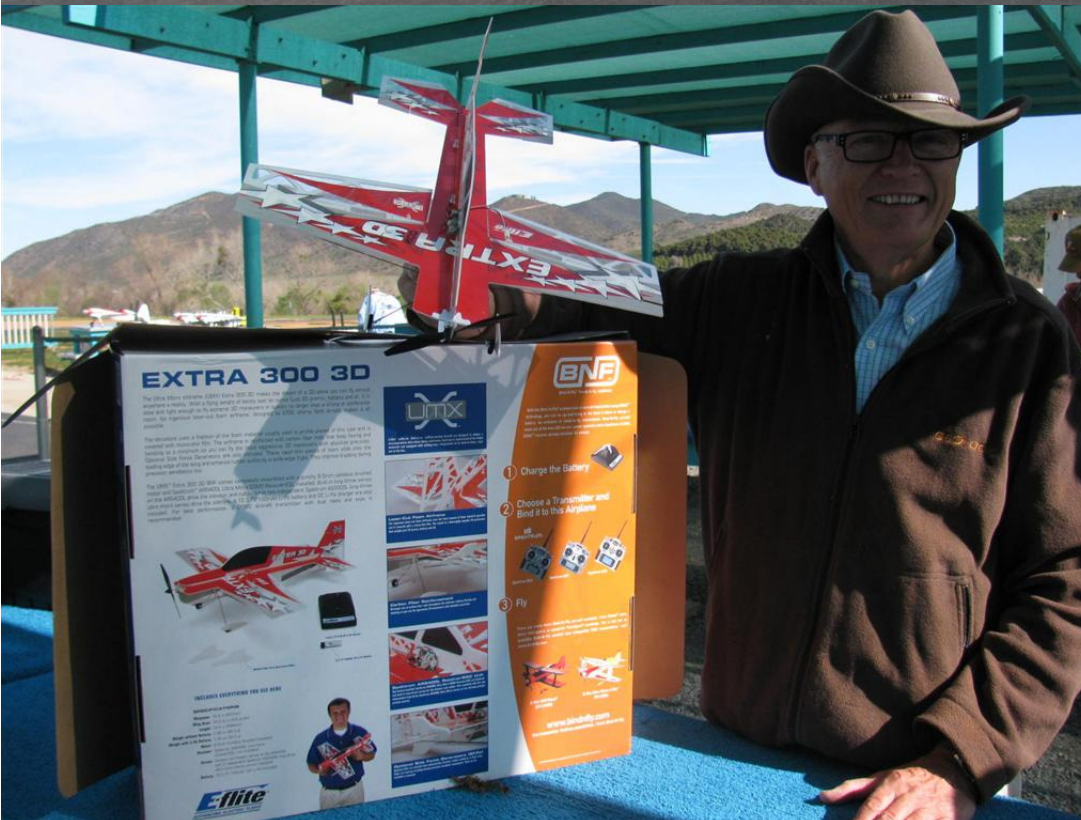
Graham Lloyd has a new electric Extra 300 from Horizon Hobby. This little flyer weighs only 1.2 oz. with a wingspan of 16.8 in. and comes entirely assembled ready-to-fly right out of the box from E-flite. It has a 12C li-po battery 1S 3.7v 150 mAh installed with 4 servos and a receiver with an ESC speed controller.
