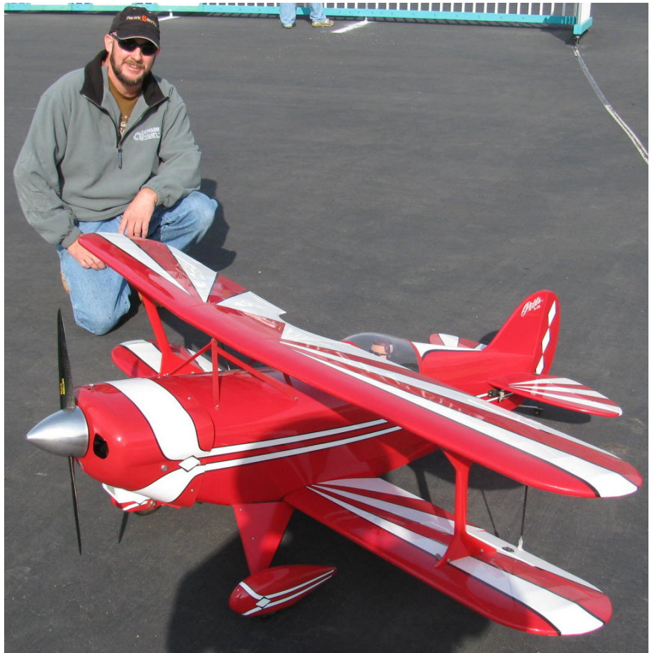
Michael Abbott is flying this Pitts S-2S biplane 1/3 scale ARF from Great Planes. It is powered by an OS-BGX 35cc glow engine. The wingspan is 68.5 in., wing area is 1303 sq. in., and it weighs 14 lbs. Ethel Burke photos
