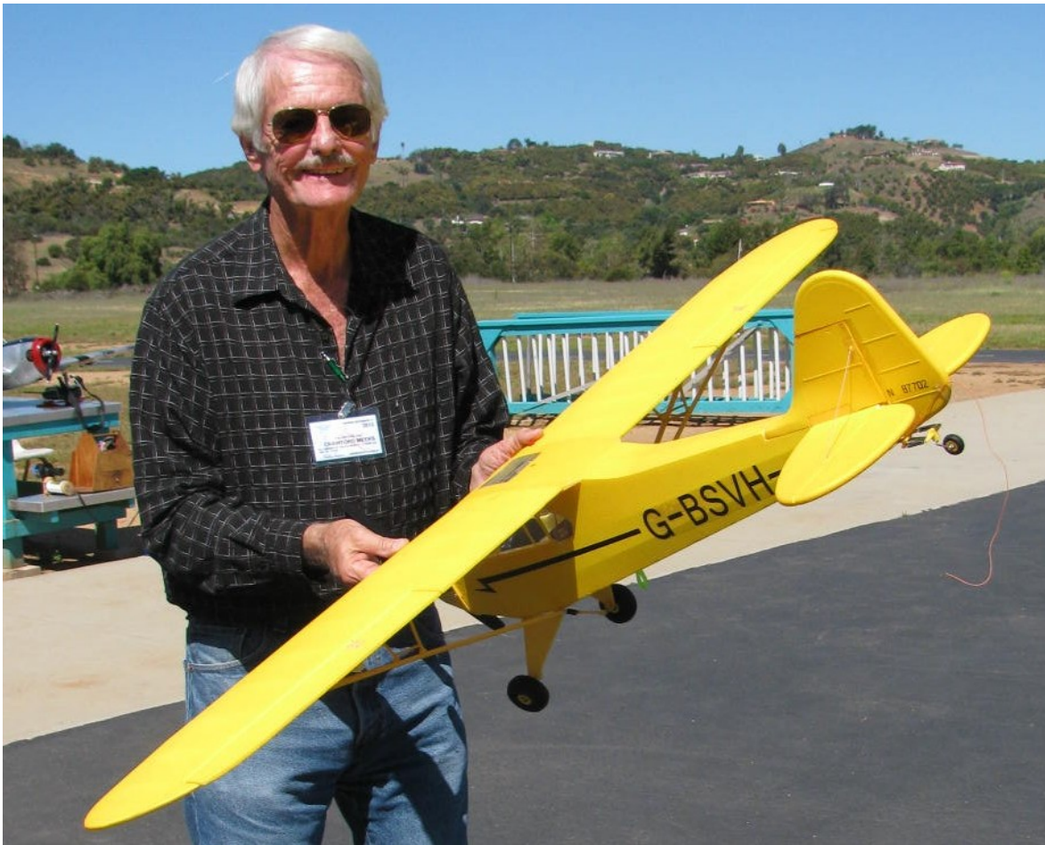
Crawford Meeks has a new Piper Cub J-3 with spring-loaded landing gear. He is running a 350 watt electric motor, 30 amp speed control, and 3S 2200 battery.
