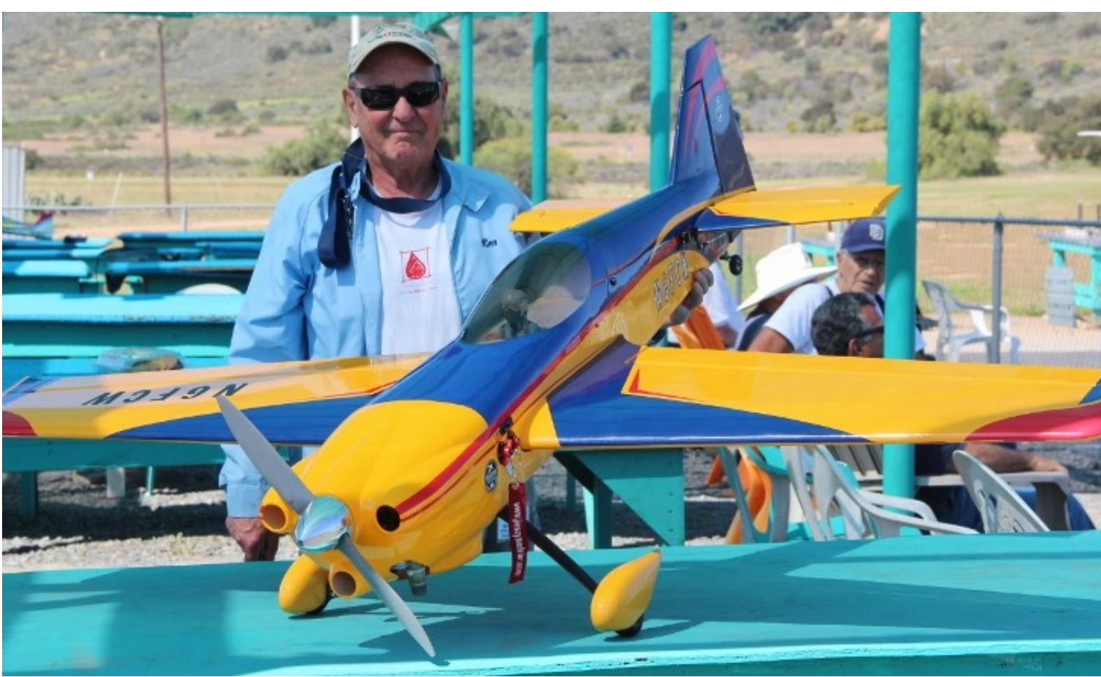
April 17, 2012 Board Member Ron Schuyler and his new 26% MXS-R in Matt Hall Colors by Peak Models, DRC-30CC Power, 75" Wing Span 69" Length DRC-30CC Power Sullivan Skywriter Smoke System, Jersey Modeler Fuel & Smoke refueling system, Carbon Fiber Landing Gear, Wing & Tail Tube, Approx. weight 11lbs (It must be helium filled!)
