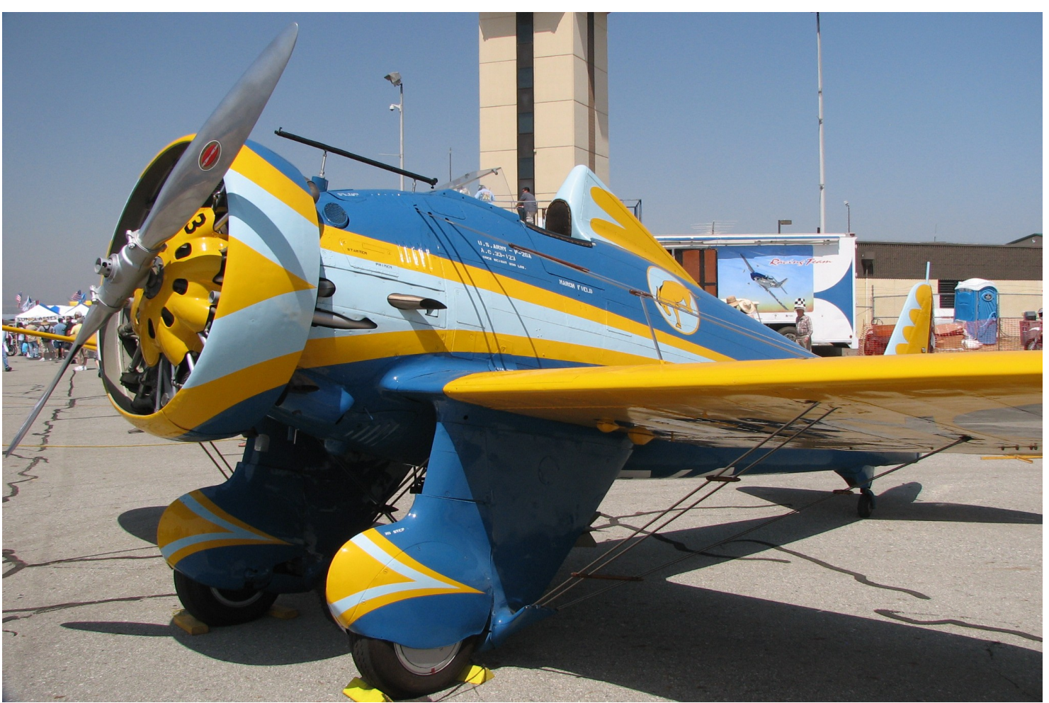
This rare P-26A is one of the last flyable planes left. It was the first all-metal pursuit plane from about 1935. The San Diego Aerospace Museum built a non-flying replica pictured below. Joe Buko photos
