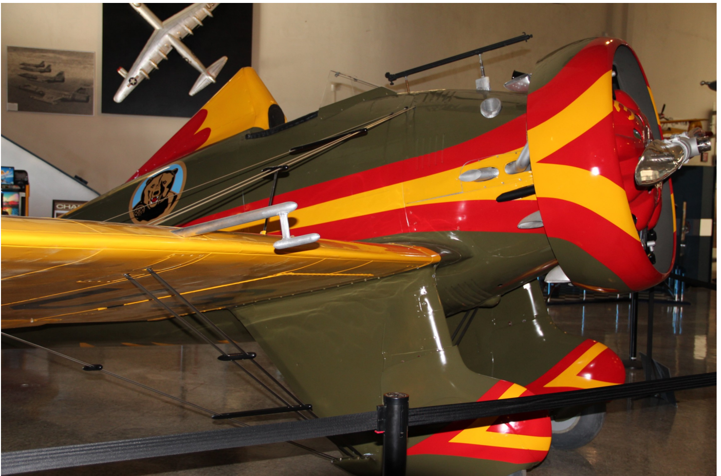
This rare P-26A is one of the last flyable planes left. It was the first all-metal pursuit plane from about 1935. The San Diego Aerospace Museum built a non-flying replica pictured below. Joe Buko photos
