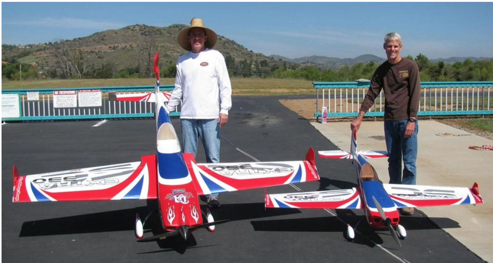
John Hartsell is flying this new Extra 330 from 3D Hobby. The wingspan is 72 in. and it has a Hacker electric motor, Castle speed control with a 6 cell 5100 mAh pack. Arnon Brouner has the big brother size with a 103 in. wingspan powered by a DA-120cc gas engine.
