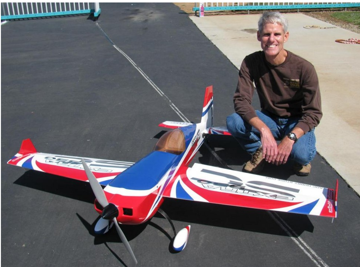
John Hartsell is flying this new Extra 330 from 3D Hobby. The wingspan is 72 in. and it has a Hacker electric motor, Castle speed control with a 6 cell 5100 mAh pack. Arnon Brouner has the big brother size with a 103 in. wingspan powered by a DA-120cc gas engine.
