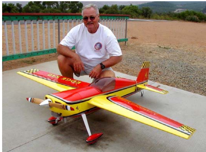
Varley Longson provides us with lots of excitement as he flies his new Edge 540 ARF by Carl Goldberg. It is powered by a DA-50 gas engine with a 23 x 8 prop. The wing span is 77 in. and he is running high-
