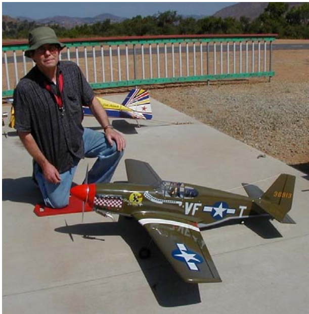
Ed Ramsey returns after an absence bringing out a new Sig ARF P-51B model razorback for its maiden flight. He runs a Saito 100 4-stroke glow engine with Spring Air retracts weighing only 9-1/4 lbs.
