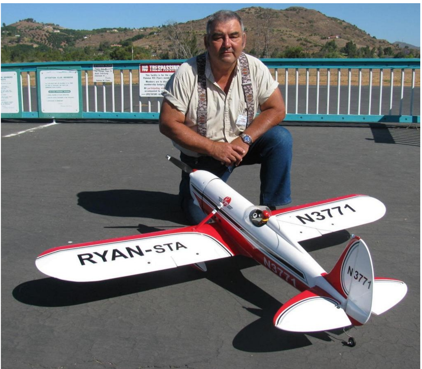
Chuck Micheli had a successful maiden flight with this new Ryan ARF from Black Horse Models. The wing-span is 70.8 in. It is powered by an OS-91 two-stroke glow engine running a 16 x 6 prop. It is flown with a JR-8103 radio.
