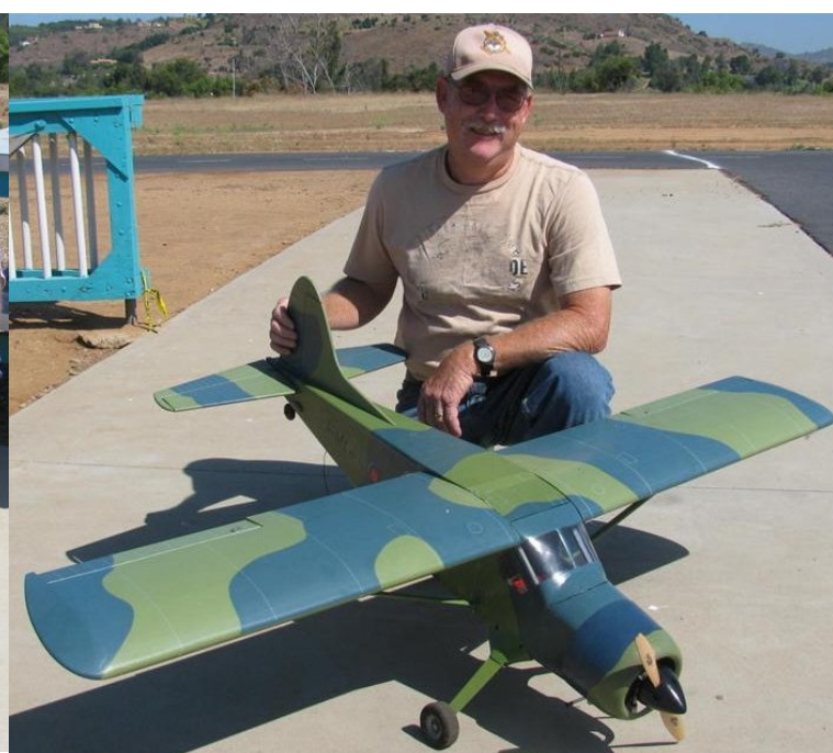
Joe Villarreal is flying this de Havilland Beaver DHC-2. It is powered by a Saito .72 four-stroke engine running a 13 x 8 prop. The wingspan is 63 in. and it weighs 6 lbs. 13 oz.
