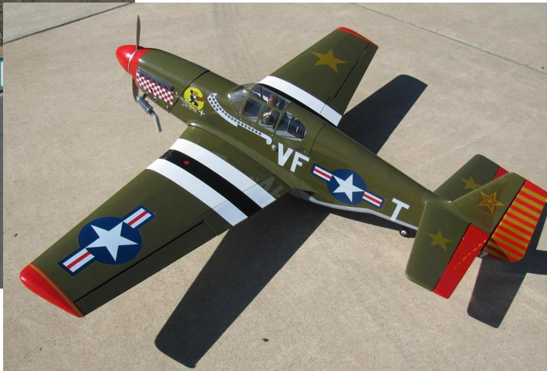
Frank Burke is flying this P-51B Mustang by Sig Models. The air frame was purchased from Ed Ramsey. It is powered by a Saito 100 four-stroke glow engine with Electro Dynamics on-board glow and uses Robart air retracts. The wingspan is 67 in. with a wing loading of 28 oz. and weighs 9 lbs. 7 oz.
