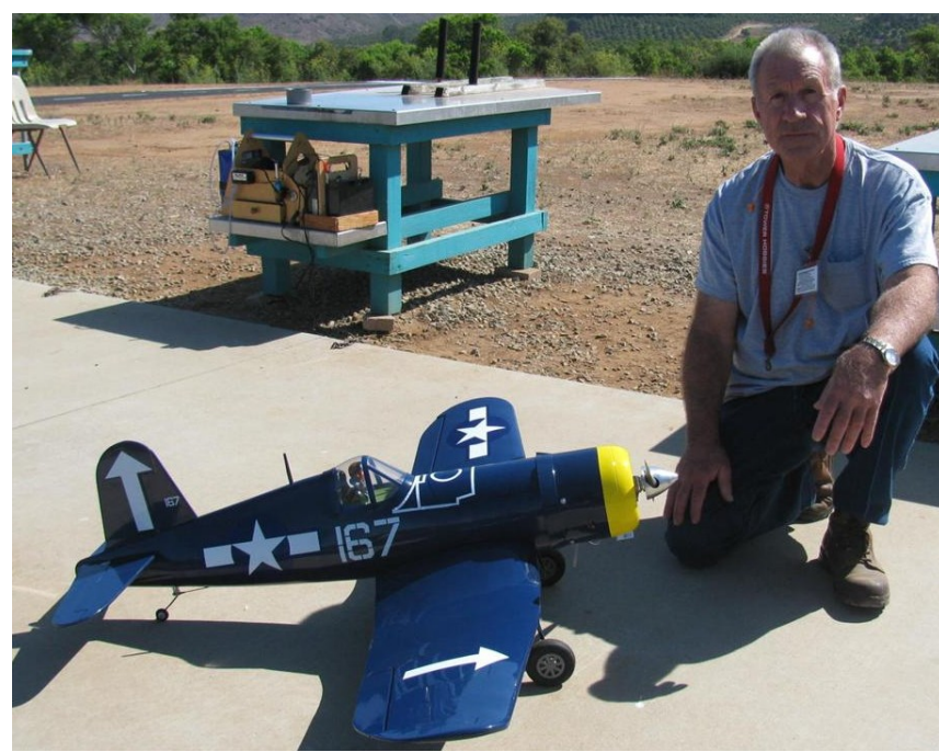
Jim Truett is flying this new Corsair from Hangar 9. It has a wingspan of 57 in; wing area is 620 sq. in.; fuselage is 45.5 in.; and it weighs 8 lbs. It is powered by a Saito 115 four-stroke glow engine running a 14 x 6 prop.
