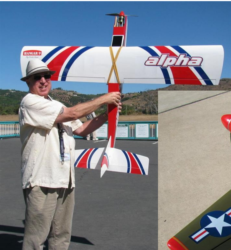
Roy DeMille has a new Alpha 40 from Hangar 9. It has a wingspan of 63 in. It flew great on its maiden flight with an electric 45 Bigfoot motor, 60 amp ESC, and 4000 mAh LiPo battery
